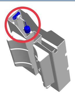
**2a.** Use scissors to remove the transparent plastic silencer tube from the valve, cut as high up as possible (just below the blue retaining ring) and take care not to drop it into the tank. Discard the silencer.
